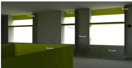
Optimize design to achieve glare free daylight with minimum external heat gains
